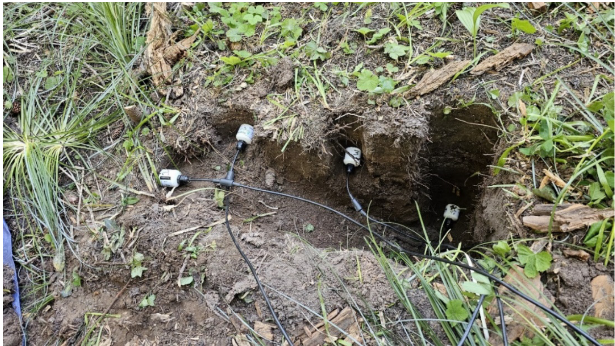
Figure 1.—Small pit used for the placement of soil moisture and temperature probes.
