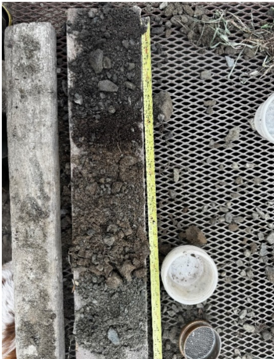
Figure 1.—A soil profile from a high tunnel. Notice the original surface buried under construction fill.
