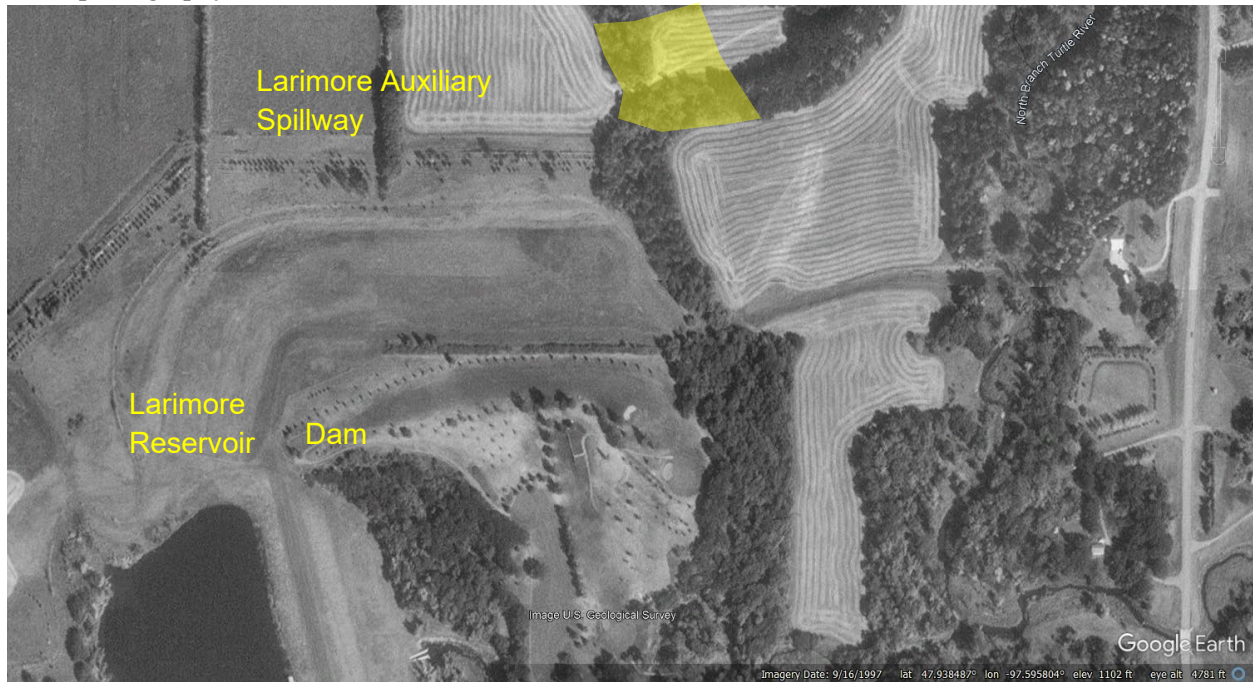
Figure 1. Google earth aerial photography dated September 16, 1997. The Pale yellow polygon represents the location of auxiliary spillway erosion and the EWP tree removal and grading repair.
