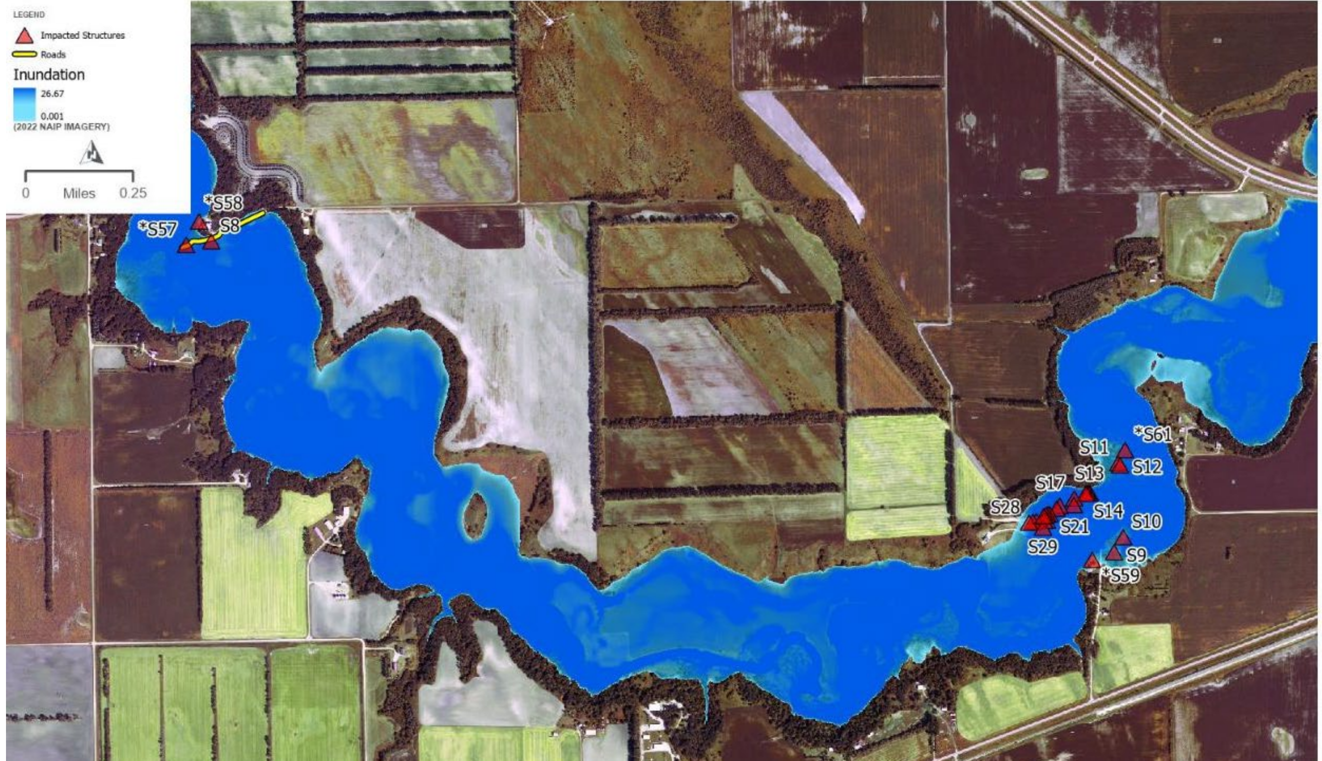
Appendix C-8: Breach Inundation, Hazard Class Analysis - 2
