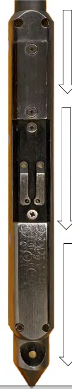
Soil Compaction, bulk density (Force sensor)
