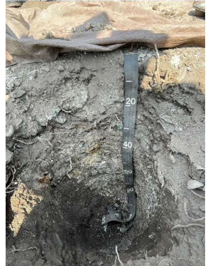
Coal ash and a thin topsoil cap in a filled marsh at a golf course in Ithaca, New York.
