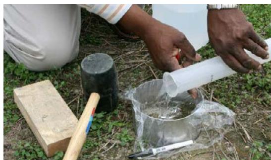
Figure 5: Preparing soil infiltration test
