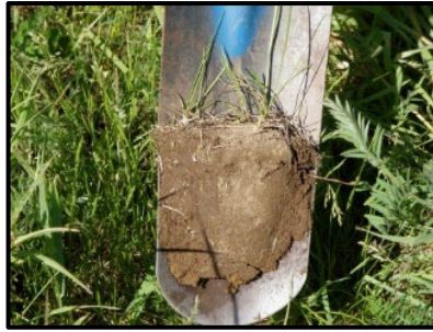
Figure 14: Using a sharpshooter to extract a slice of soil
