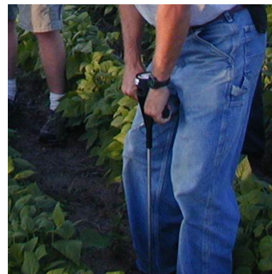
Figure 6: Applying slow, steady pressure when pushing penetrometer into soil
