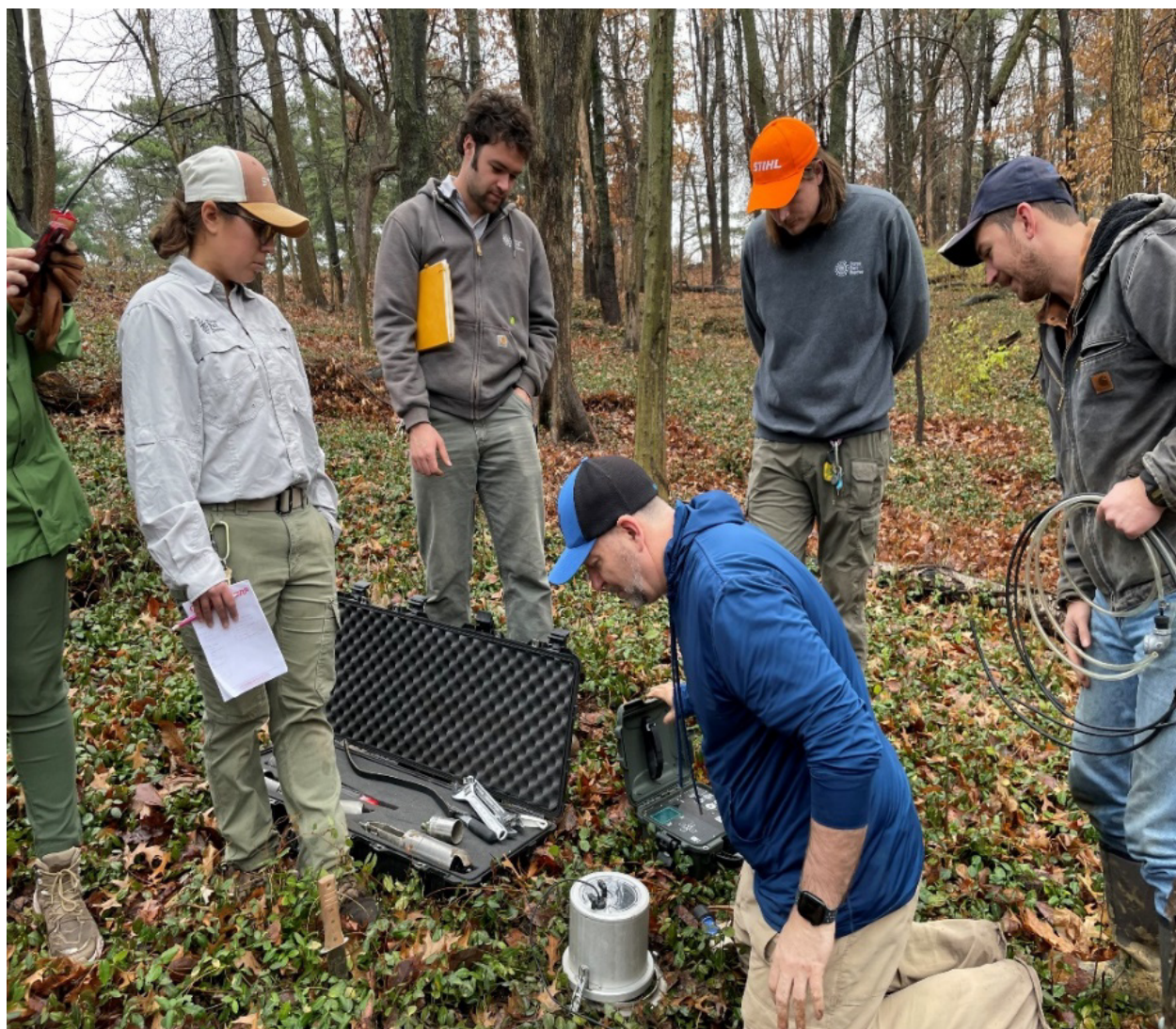
Figure 1.—SSO Leader Ralph Tucker (lower middle) and Soil Scientist Ryder Anderson (far right) demonstrate the use of infiltrometers and bulk-density slide hammers for FPF staff.
