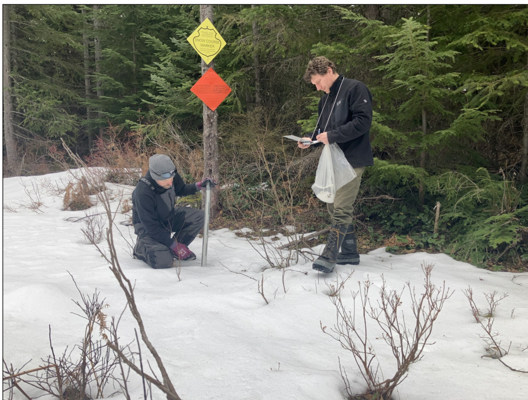
Scott Pries, Tacoma Watershed Inspector, and Tyler Traweek, Tacoma Water Environmental Specialist, measure Grass Mtn. No. 2 Snow Course. Snowpack is 32% of normal on February 1.
