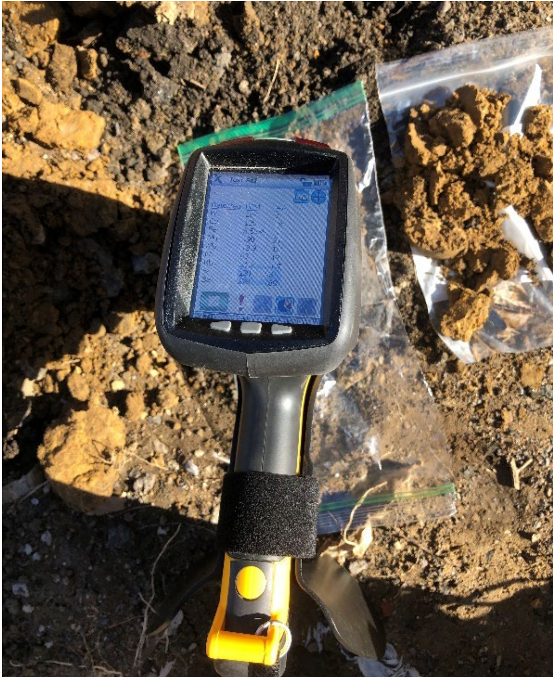
Figure 3.—Taking a pXRF measurement in the field on an urban lot on Hartford, CT. The plastic bag protects the sensor during operation.
