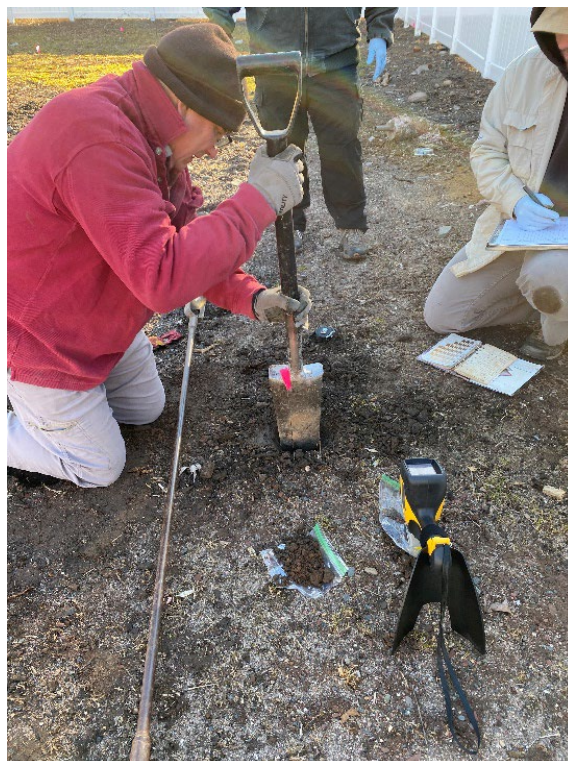
Figure 1.—Donald Parizek, Special Projects Office soil scientist, excavates a soil pit in preparation for pXRF analysis in the field.
