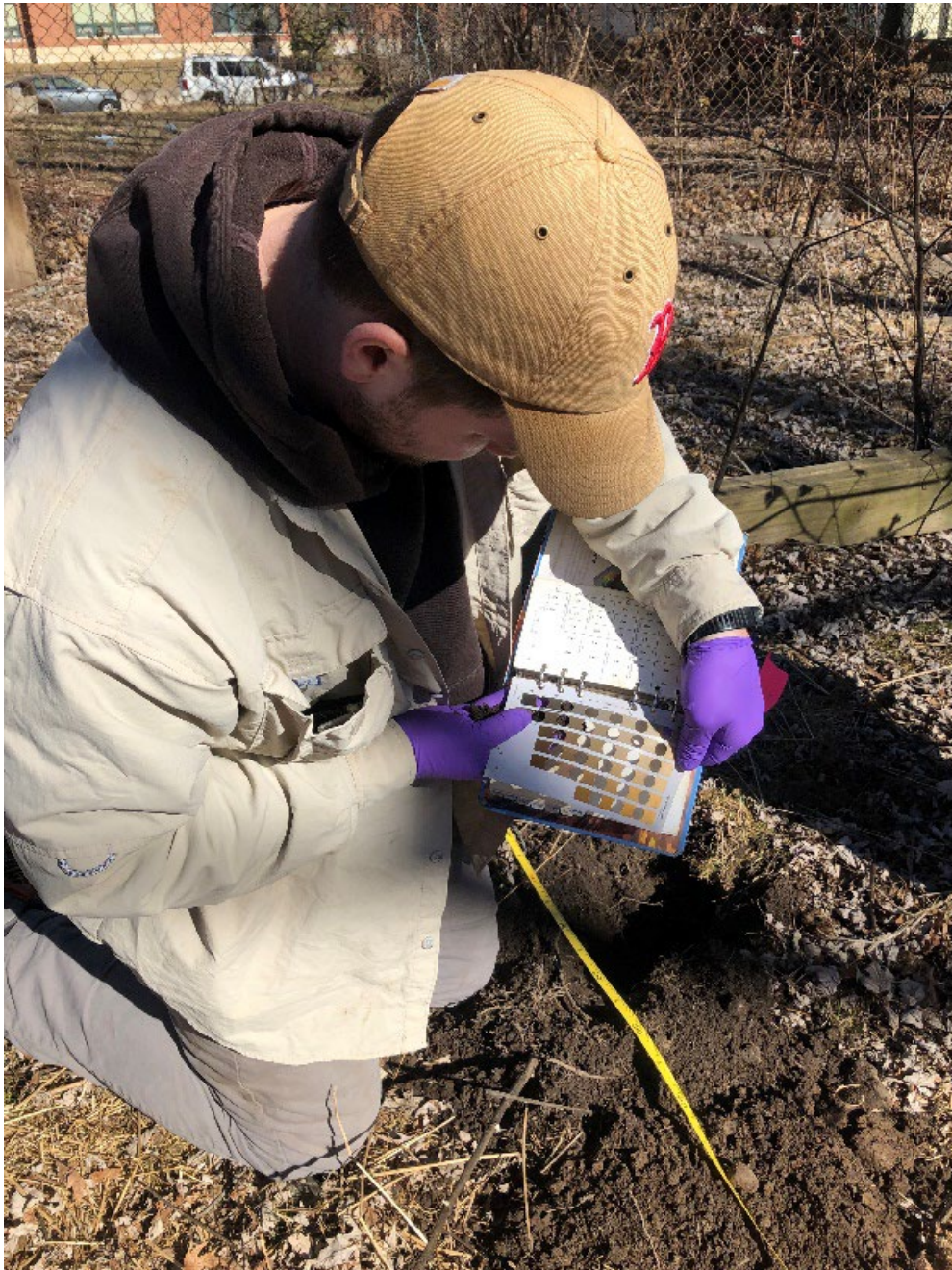
Figure 4.—Braden Fleming, Special Projects Office soil scientist, wears nitrile gloves for safety while identifying soil color on an urban lot in Hartford, CT. Hand texturing soils is more challenging while wearing gloves.
