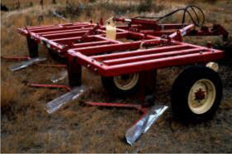
Figure 10. The blade plow or sweep plow undercutter terminates cover crops and weeds by severing root crowns just below the surface, leaving residues in place and most of the soil profile undisturbed. This tool requires just the right soil moisture level, as wet conditions allow the vegetation to regrow, while very dry conditions prevent the tool from penetrating sufficiently to kill the cover crop. “It works about 50% of the time for terminating the green fallow,” Doug said. “My fallback option is the speed disk.” Photos by Drew Lyon, U. Nebraska.
