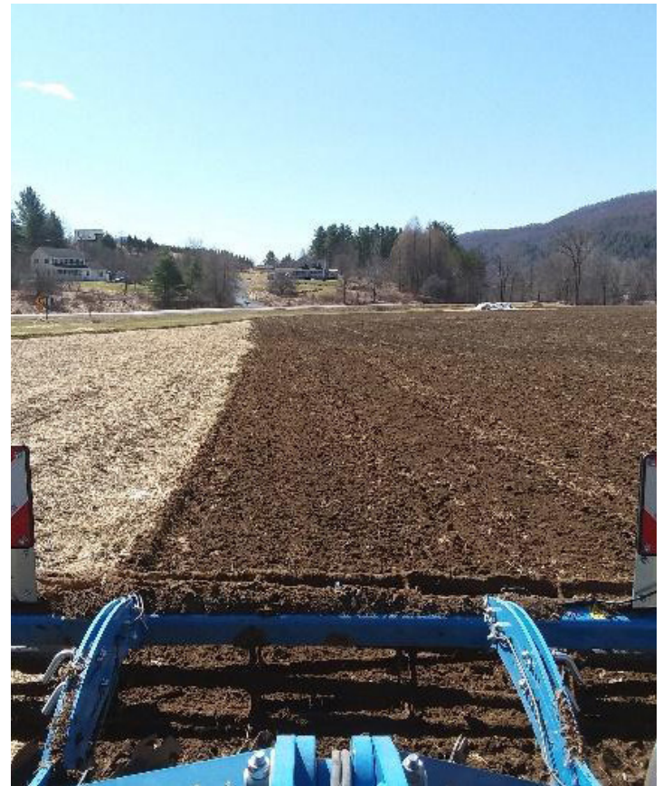
Figure 6. For most tillage operations, Burnt Rock Farm uses a 2.5 meter (8 ft) Farmet Softer high-speed disk equipped with independently sprung, compound-angled, notched disks and a depth-setting rolling basket in the rear. Working 3-4 inches deep at a forward speed of 7-8 mph, the disk chops and incorporates flail-mowed cover crops (left) and makes a satisfactory bed for transplanting in two passes 10 days apart. Winter-killed cover crops require only one pass (right). Because the disk works best in moist soil, Justin incorporates mid-summer covers after a rainfall.
