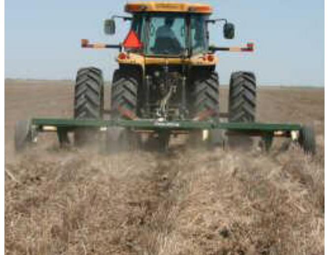
Figure 10. The blade plow or sweep plow undercutter terminates cover crops and weeds by severing root crowns just below the surface, leaving residues in place and most of the soil profile undisturbed. This tool requires just the right soil moisture level, as wet conditions allow the vegetation to regrow, while very dry conditions prevent the tool from penetrating sufficiently to kill the cover crop. “It works about 50% of the time for terminating the green fallow,” Doug said. “My fallback option is the speed disk.” Photos by Drew Lyon, U. Nebraska.
