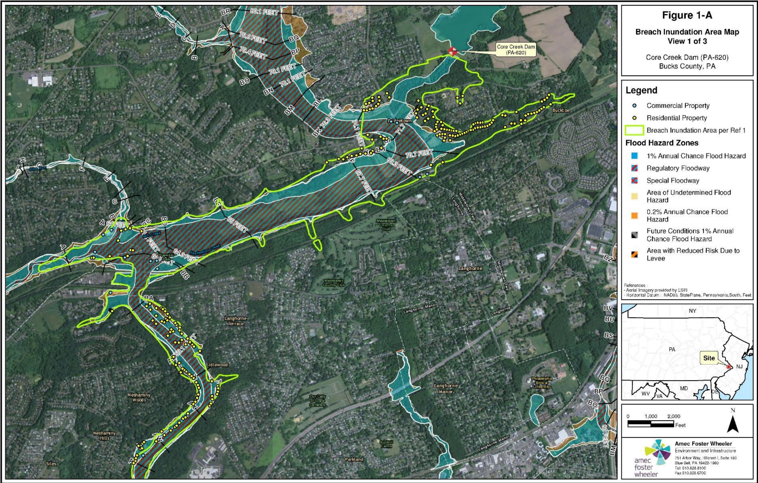
Figure C-8A Core Creek Dam (PA-620) Breach Inundation Map
