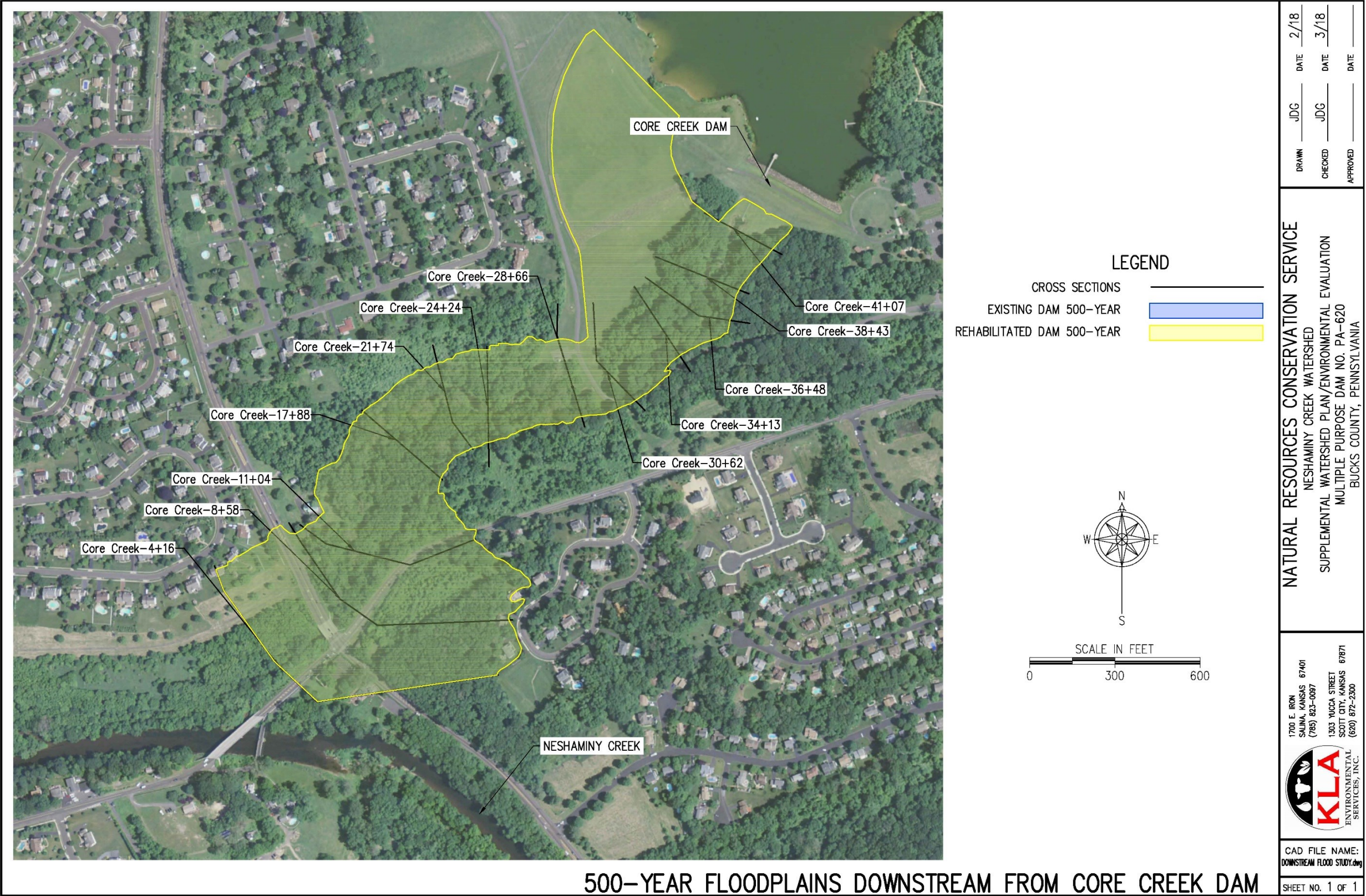
Figure C-10C Core Creek Dam (PA-620) Existing and Rehabilitation Frequency Flood – 500-Year
