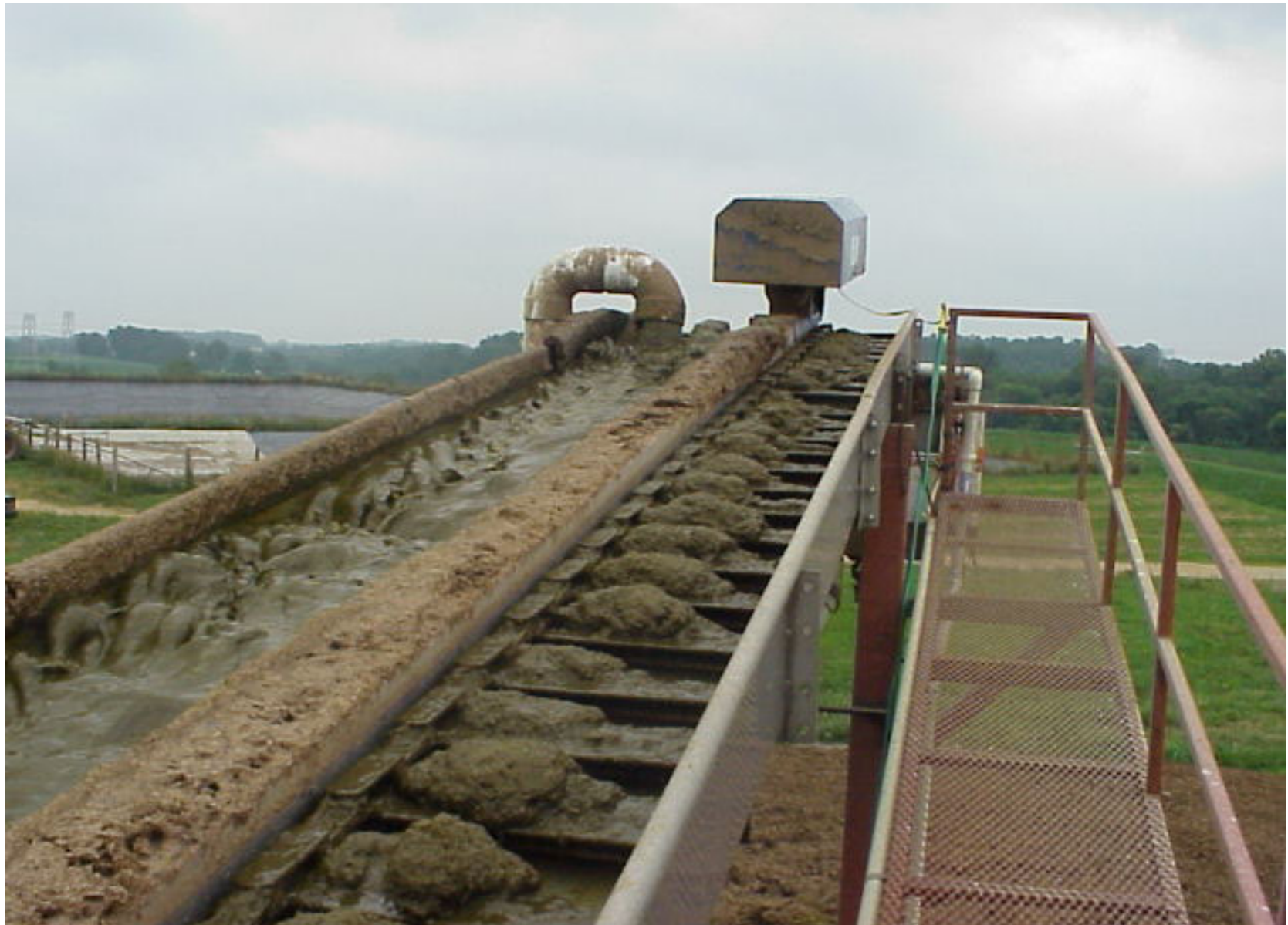
Manure Solids separation with Albers gravity screen system
