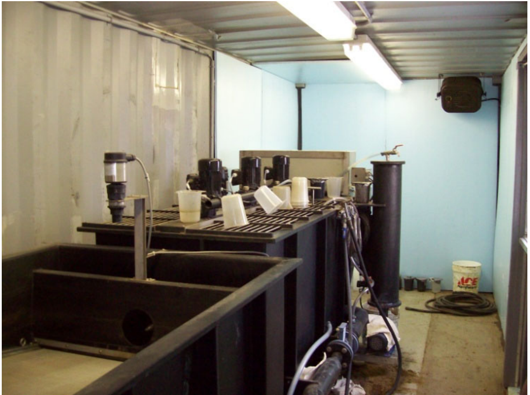
Removing manure solids by adding a “flocculent” to consolidate solids
