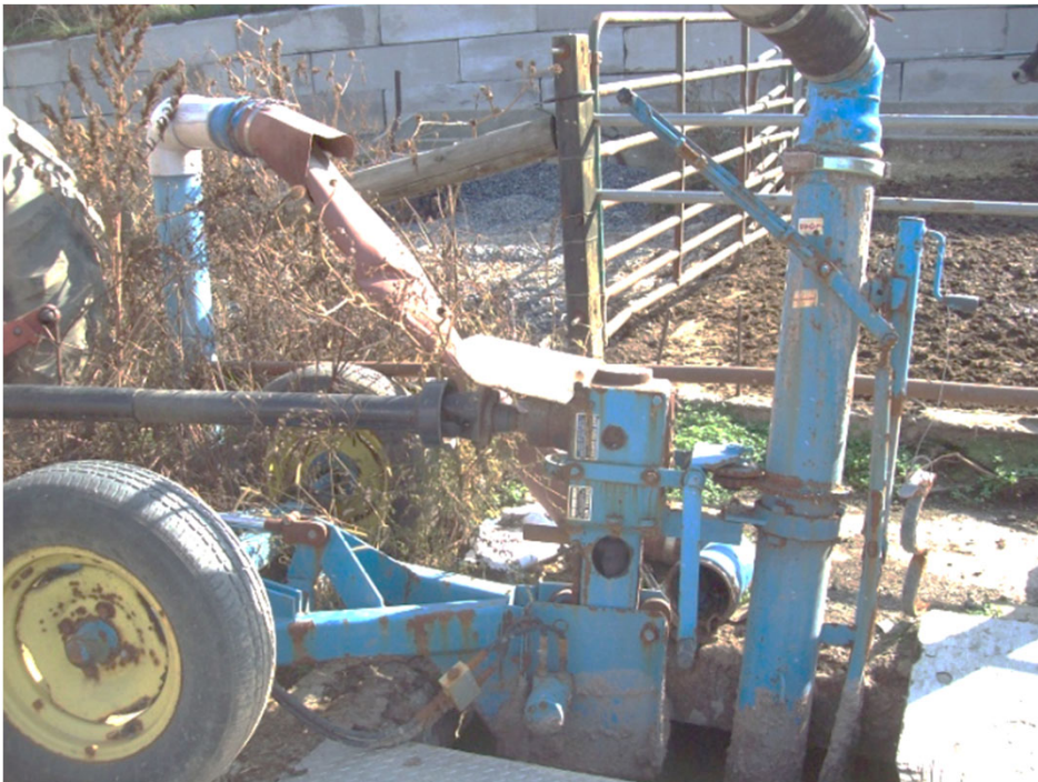
PTO driven manure pump to transfer manure from short- term storage to long-term storage
