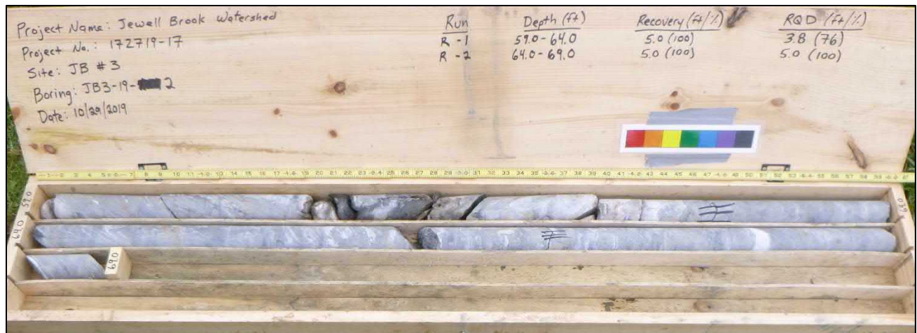
Test Boring JB3-19-2 Box: 1 of 1 Depth: 59.0' to 69.0' Condition: Dry Date: October 29, 2019
