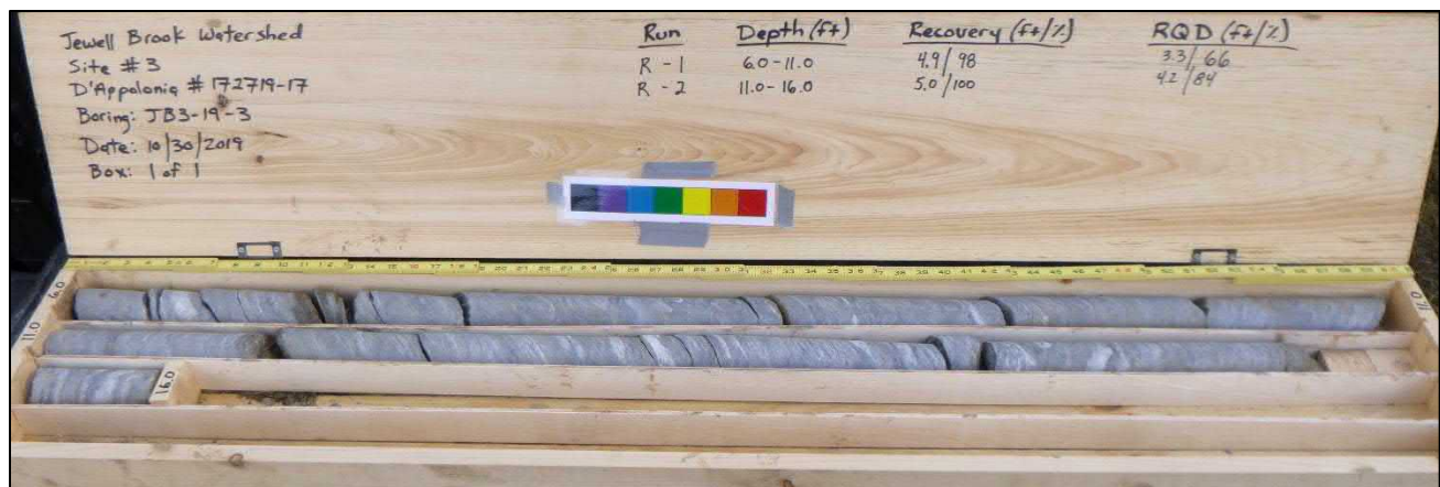
Test Boring JB3-19-3 Box: 1 of 1 Depth: 6.0' to 16.0' Condition: Dry Date: October 30, 2019
