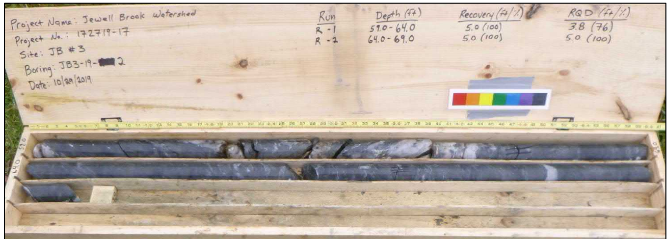
Test Boring JB3-19-2 Box: 1 of 1 Depth: 59.0' to 69.0' Condition: Wet Date: October 29, 2019
