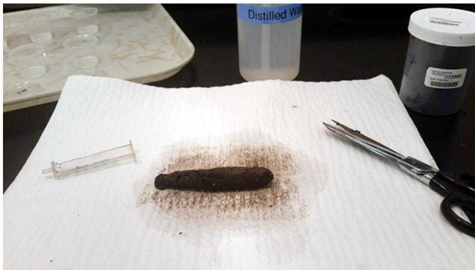
Figure 5B–1.—Sample preparation. Sample fibers are cut into 0.5- to 1.0-cm long segments.
