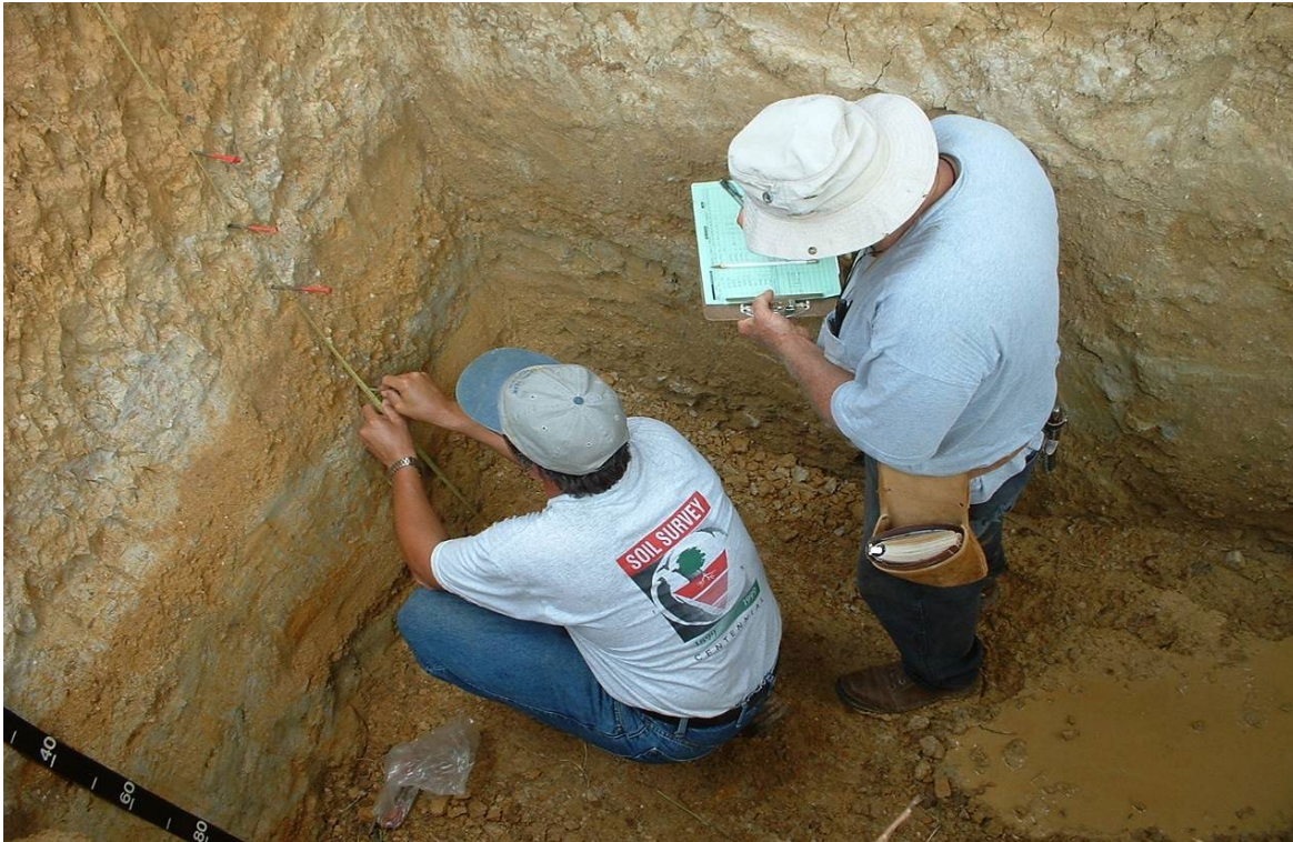
Figure 1A-3.—Soil horizons or zones of uniform morphological characteristics are identified for sampling.
