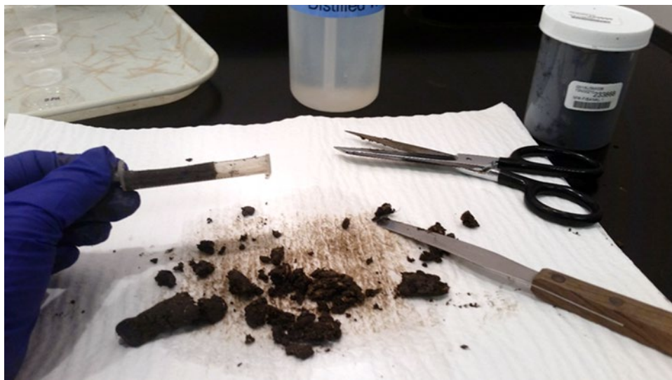
Figure 5B-2.—Sample preparation. Sample segments are packed in syringe.
