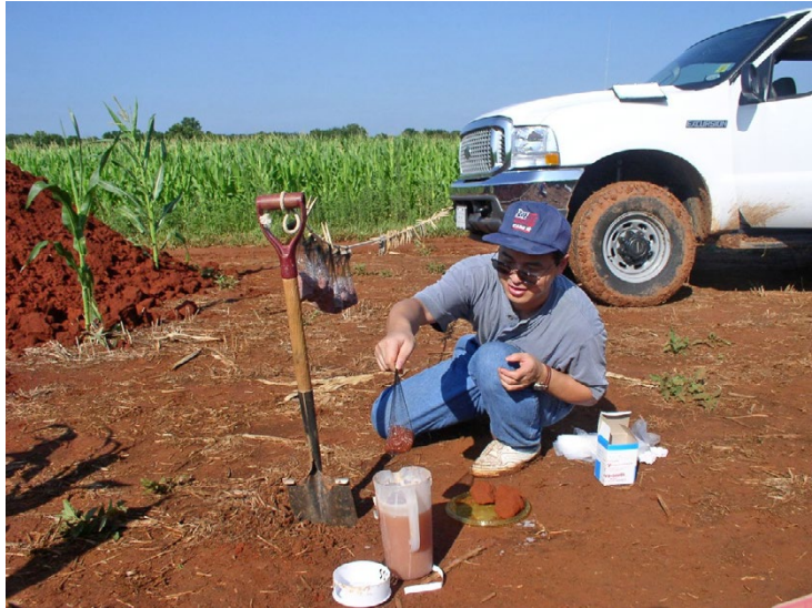
Figure 3B1b-1.—Dipping clods with hairnet in plastic lacquer.
