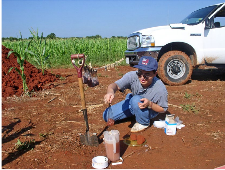
Figure 3B1a-1.—Dipping clods with hairnet in plastic lacquer.
