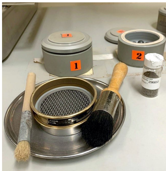
Figure 1B1b2d-2.—Bowls, balls, and sample vial used with planetary ball mill.
