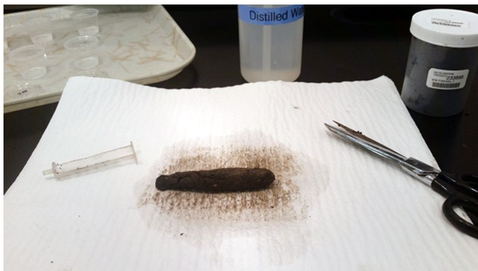
Figure 4C1a1a4-1.—Sample preparation. Sample fibers are cut into 0.5- to 1.0-cm long segments.
