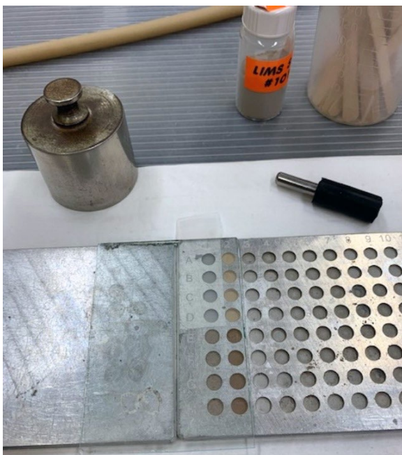
Figure 7A7-10.—First two columns protected against cross-contamination with glass plate.
