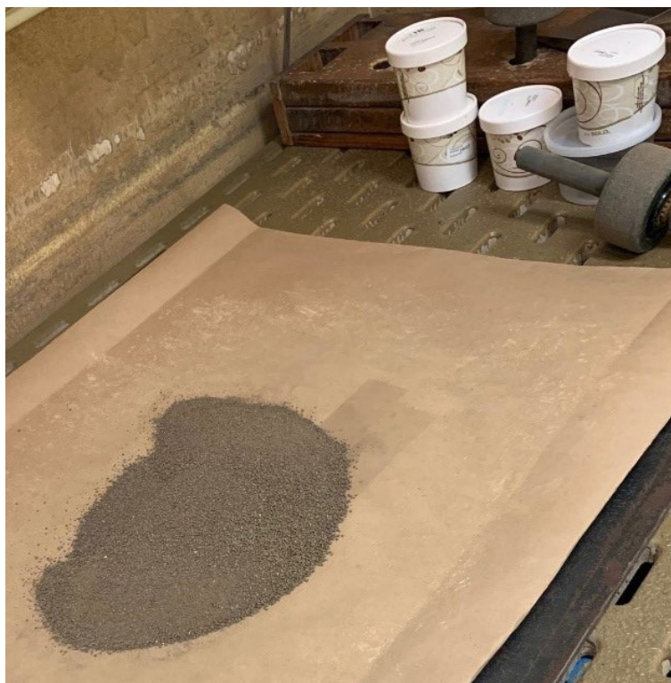
Figure 1B1b2b–6.—Homogenized <2-mm processed soil sample ready for subsampling.
