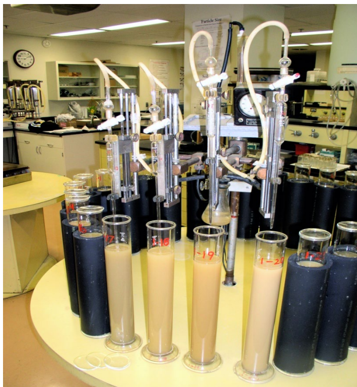
Figure 3A1a1-3.—Shaw Pipette apparatus and Lowy Pipettes used for particle-size analysis at the USDA–NRCS Kellogg Soil Survey Laboratory.
