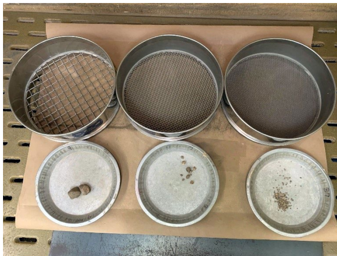
Figure 1B1b2b–5.—Rock fragments collected during sieving; collect weight of each size fraction after grinding soil sample is complete.
