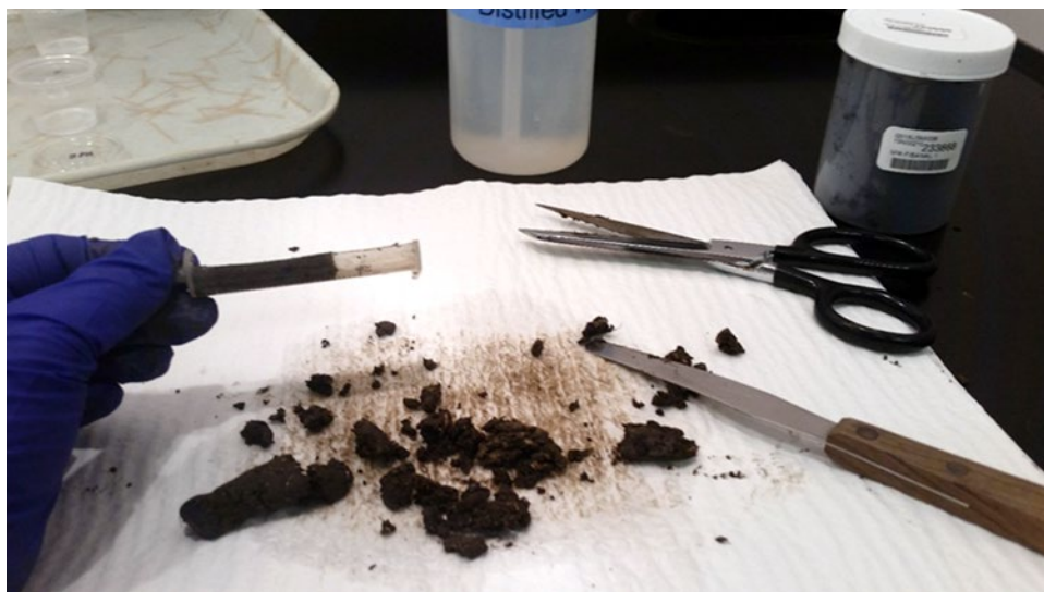
Figure 5C–3.—Sample preparation. Sample segments are packed in syringe.
