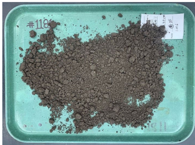
Figure 1B1b2b–3.—Sample prepared for drying with tared tray and sample tag.
