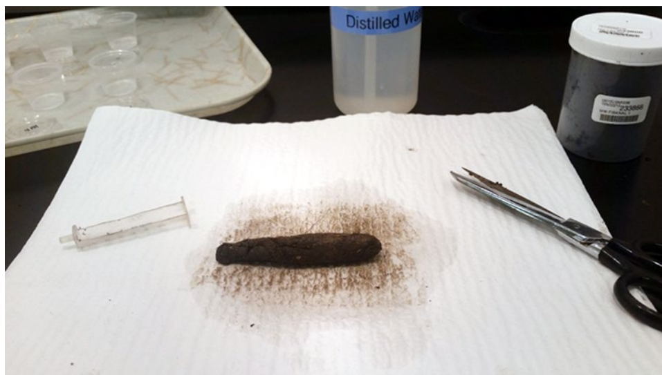
Figure 5C–2.—Sample preparation. Sample fibers are cut into 0.5- to 1.0-cm long segments.
