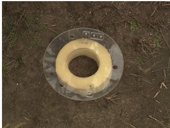
Figure 3B3a-1.—Plexiglass ring assembly.
