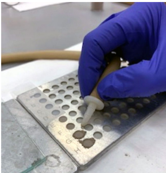
Figure 7A7–6.—Vacuuming excess sample from around wells.
