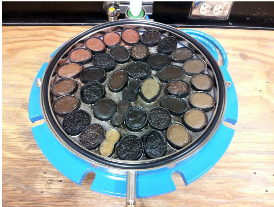
Figure 3C2b-2.—Sieved (<2-mm) soil placed in pressure-membrane extractor.
