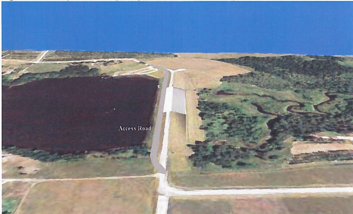
Figure 6. Example of RCC Spillway with Access Road on Upstream Side of Embankment
